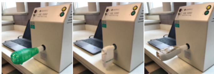
Figure 2. (L to R) Acapella, Aerobika, and vPEP attached to the IngMar ASL 5000 for performance testing
